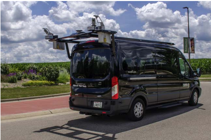
Figure 2.19 Mandli's LiDAR and pavement condition collection vehicle.
